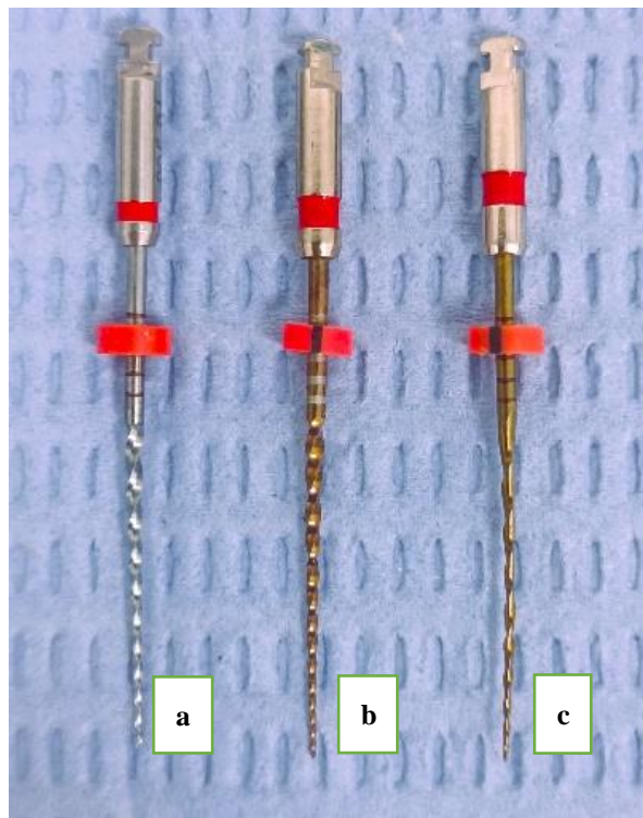
Figure 1. NiTi rotary files (a) Group 1-Orodeka Plex V, (b) Group 2- Super Flexi File Gold and (c) Group 3- Fury L60.
