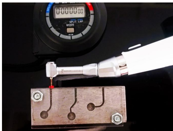
Figure 2. Setup of custom fabricated cyclic fatigue device.
